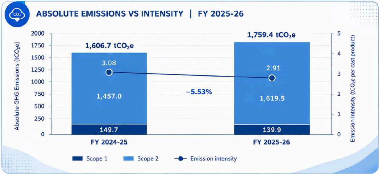
Figure E-4. Absolute Scope 1 + Scope 2 GHG emissions (stacked bars, left axis) and emission intensity per tonne of cast product (line, right axis), FY 2024-25 to FY 2025-26. Absolute emissions rose with production volume; intensity declined 5.53%.
