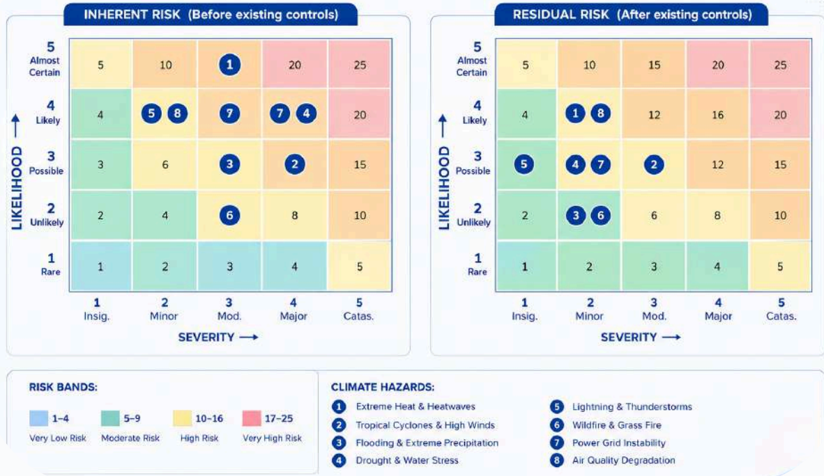
Figure C-1. Climate physical risk heat map for the Hadamtala manufacturing facility and the Kolki captive solar plant. The left panel plots the inherent risk of each of the eight identified hazards on the 5x5 likelihood-severity matrix; the right panel plots the residual risk after the application of existing engineered, procedural and financial controls. The migration of hazards from the high (orange) and moderate (yellow) bands towards the low (green) band evidences the effectiveness of the existing control architecture.
